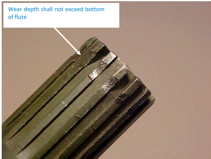
Igniter Tip Flute Wear Limits
